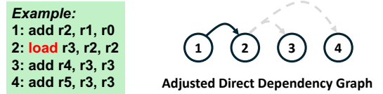
Fig. 5: Adjust the dependency graph when handling load instructions in the rename stage.
